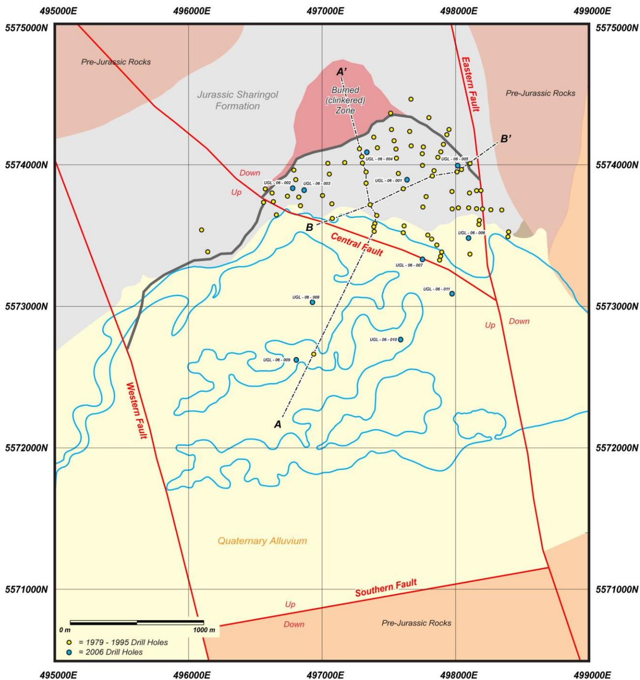
Figure 11.1 - General Geology of the Ulaan Ovoo Coal Deposit
